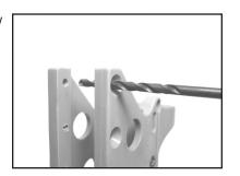
5. Carefully remove the slide assembly from the frame, making sure not to move the sight from its clamped position. DO NOT drill the frame without removing the slide assembly. Also, check to be sure you are not going to drill into the frame rail / bridge area.
