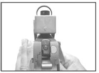
7. Remove the mounting screws and remove the sight from the frame. Now clearance drill the mounting holes in the sight with a .125" (1/8") drill or reamer.
