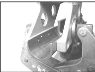
8. Degrease the mounting screws and the tapped holes in the dust cover. Install the sight using Loctite 271 or 2760 (red) on the threads of the mounting screws. DO NOT use excessive force in tightening the mounting screws. Over torquing them can fracture the mounting pads. Moderately snug is sufficient.
