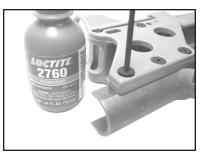
6. With the sight clamped in position, drill the front and rear mounting holes on each side using a #39 drill. Then tap the four holes you just drilled with a 5-40 tap and carefully install the mounting screws with the 5/64 allen wrench. Snug the four mounting screws and remove the clamp. Now repeat the drilling and tapping for the two remaining mounting holes.
