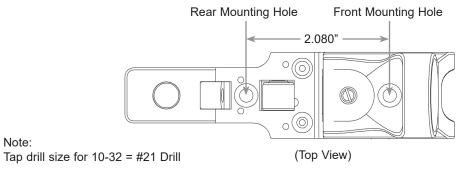
2) Using the 10-32 cap socket screws provided, secure the sight to your base. DO NOT OVERTIGHTEN! Firmly snug is sufficient (15-20 In Lbs). Applying Blue Loc-Tite to the mounting screws will prevent the sight from loosening under recoil.
